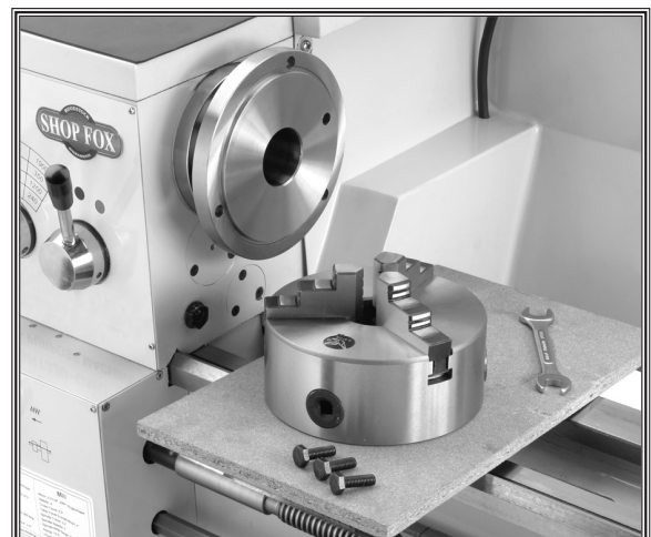
Figure 16. Chuck, hex bolts, and spindle flange.
